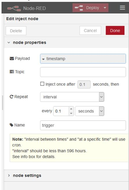
Figure 25: Node: “trigger”
