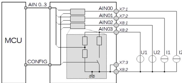
Figure 7: Setup of analog inputs
