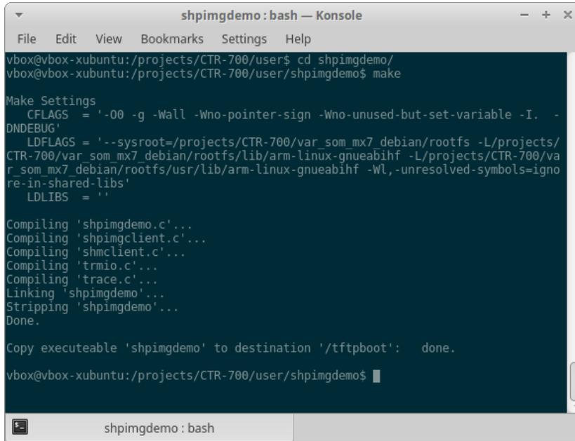
Figure 39: Generating the demo project "shpimgdemo" in the Linux development system
