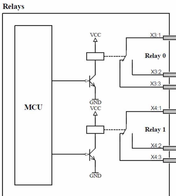
Figure 6: Setup of Relay outputs
