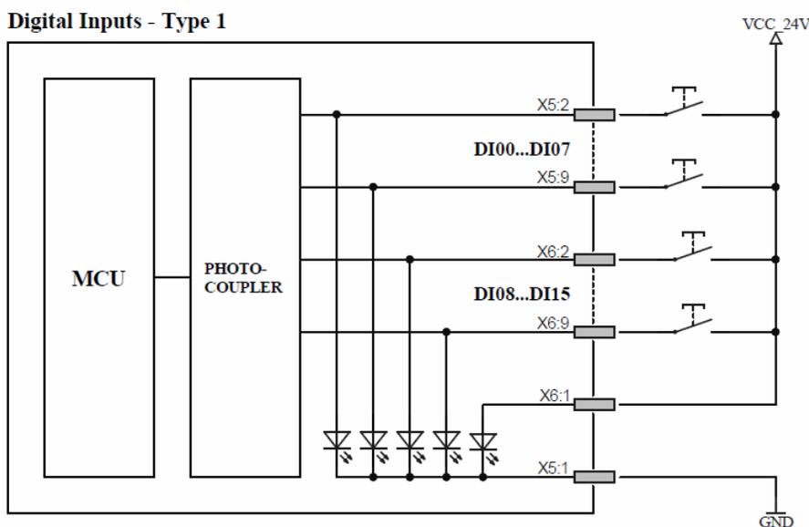
Figure 4: Setup of digital inputs
