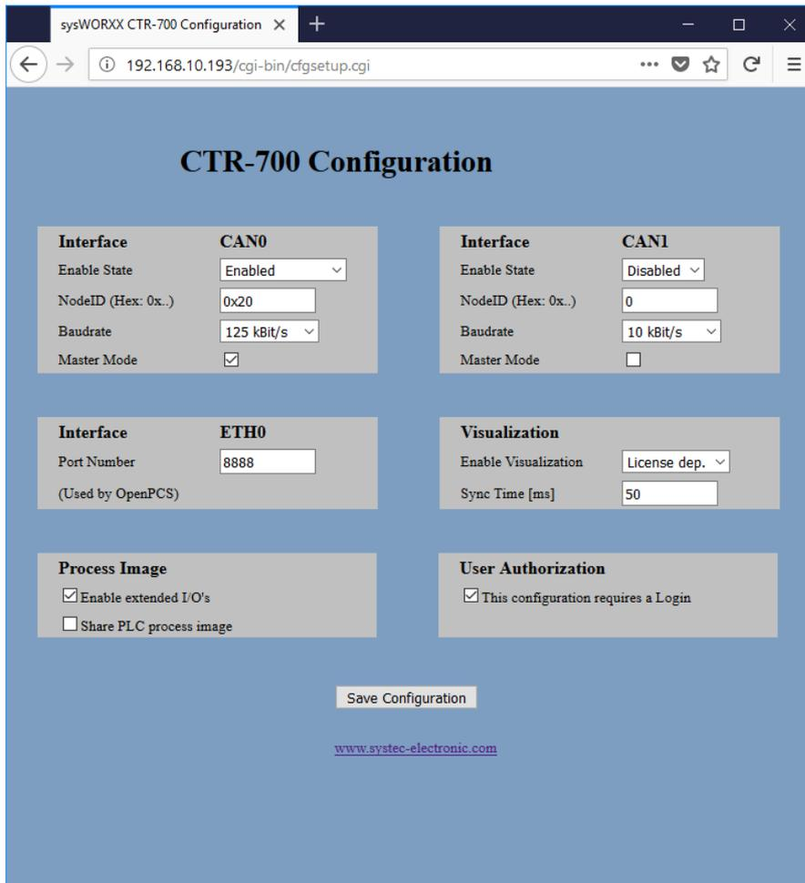
Figure 12: PLC configuration via WEB-Frontend
