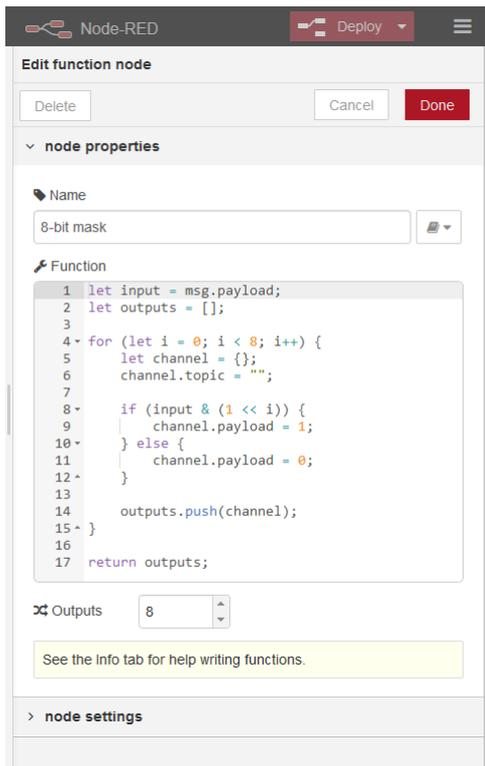
Figure 27: Node: “8-bit mask”
