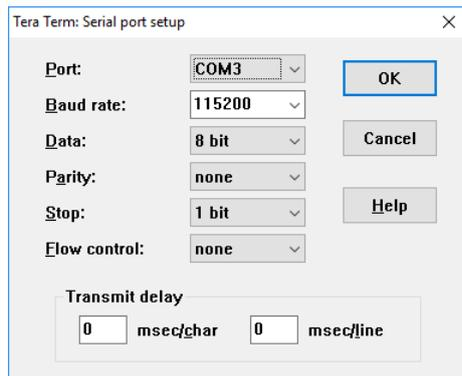
Figure 8: Terminal configuration using the example of "TeraTerm"
