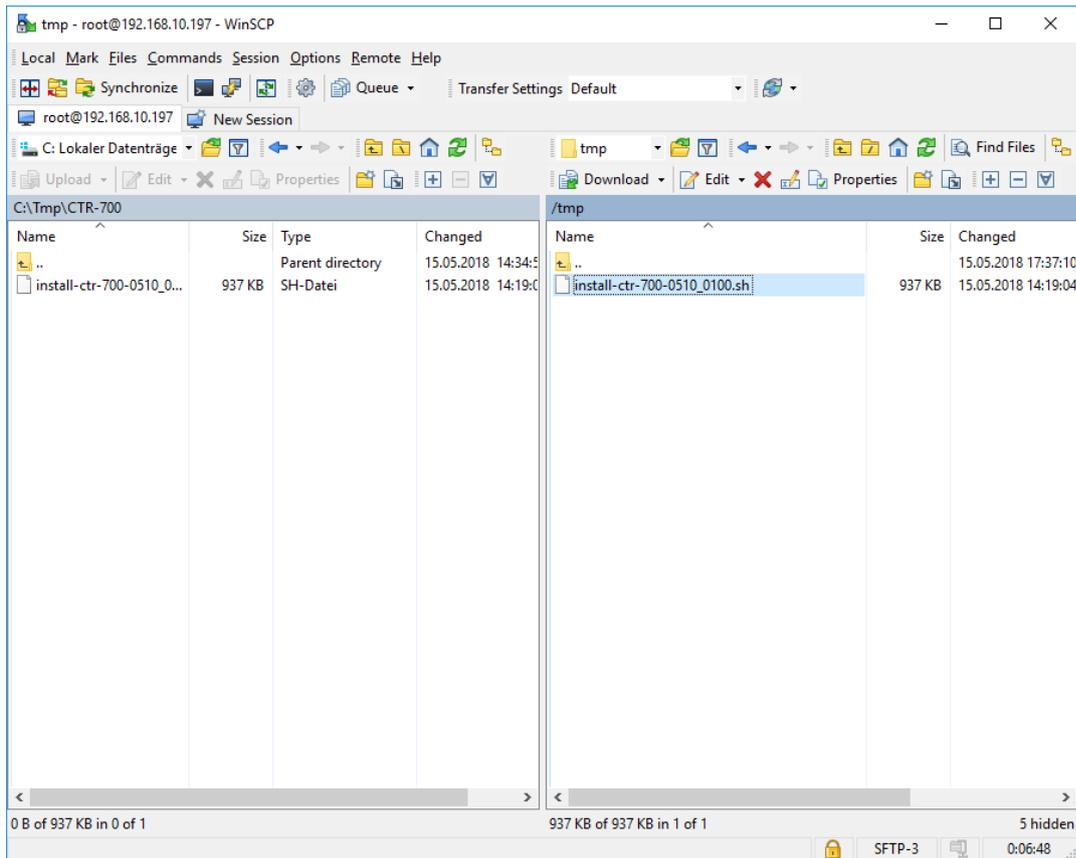
Figure 20: File transfer in SFTP client "WinSCP"
