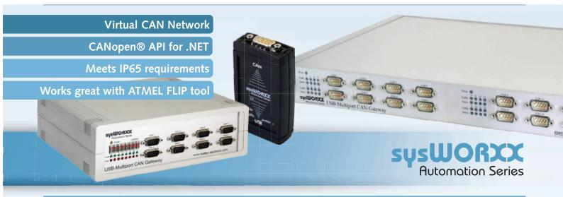
Our USB-CANmodul series provides you with an ideal solution for connecting CAN to your notebook, desktop or industrial computer. Powered by a fast 32-bit CPU, the USB-CANmodul is available with up to 16 CAN channels. The enclosed software driver is capable of simultaneously operating multiple USB-CANmodul devices with up to 64 CAN channels in total. For mobile and off-road applications we offer a rugged version with IP65 housing and connectors.
