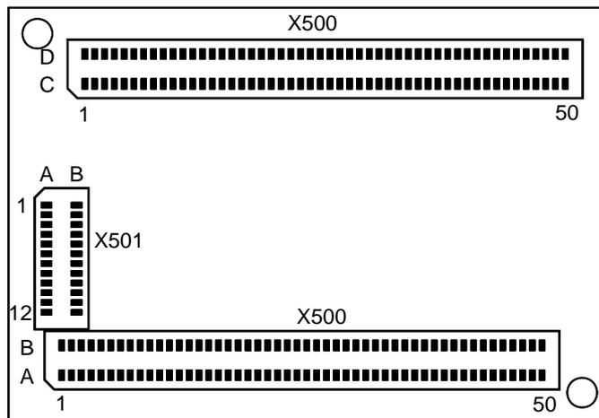
Figure 6: Pinout (top view)
