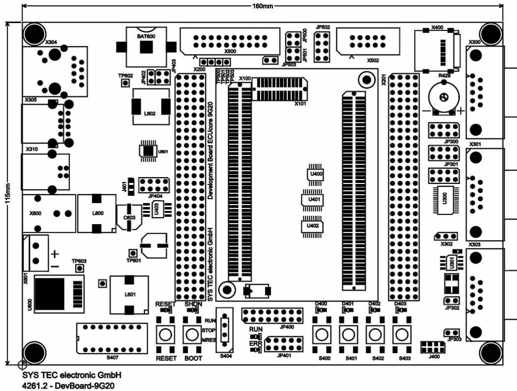
Figure 3: Positions of components
