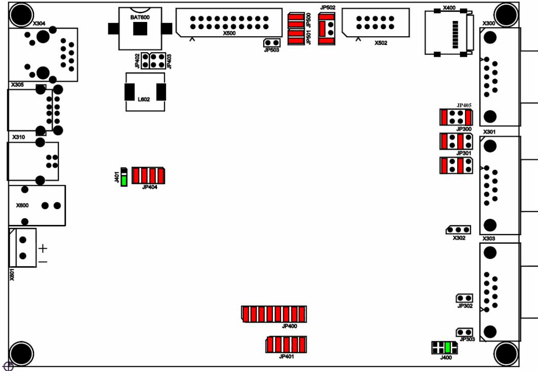
Figure 4: Default Jumper configuration
