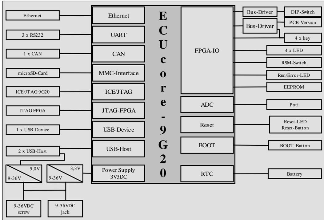
Figure 2: Block Diagram Development Board ECUcore-9G20
