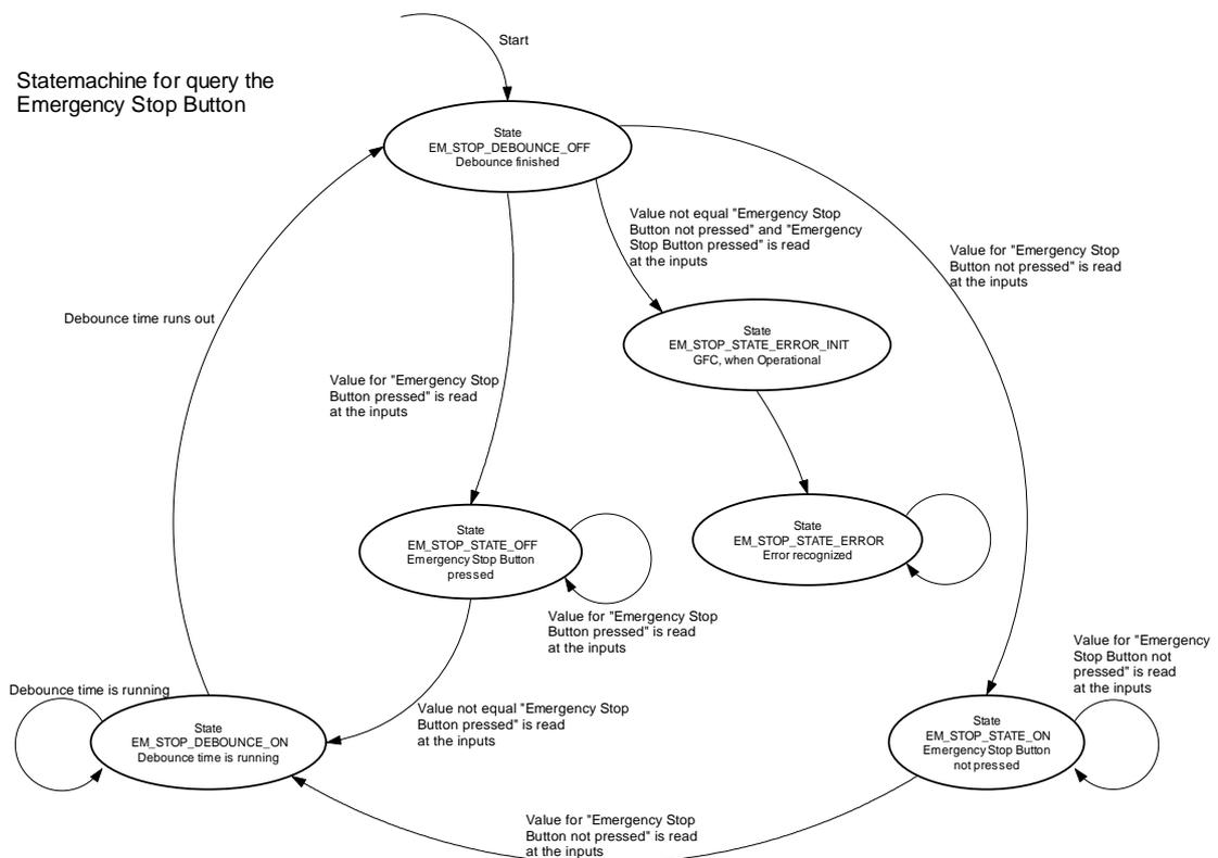
Figure 4: State Machine for Querying the Emergency Shutoff
