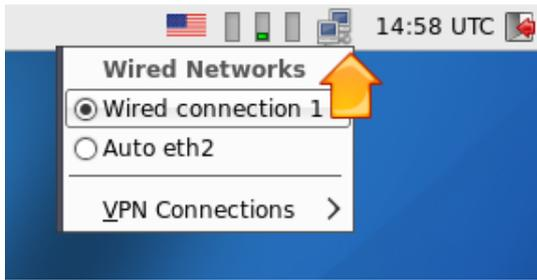
Figure 41: Changing the network configuration in the "Network Manager"
